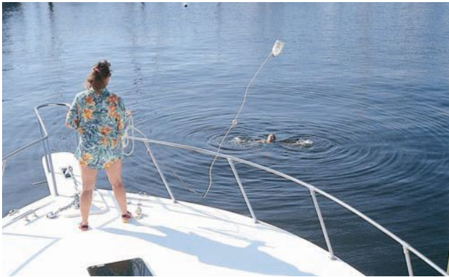
Figure 20-9 A heaving jug is a simple homemade device that can be thrown to a victim.
